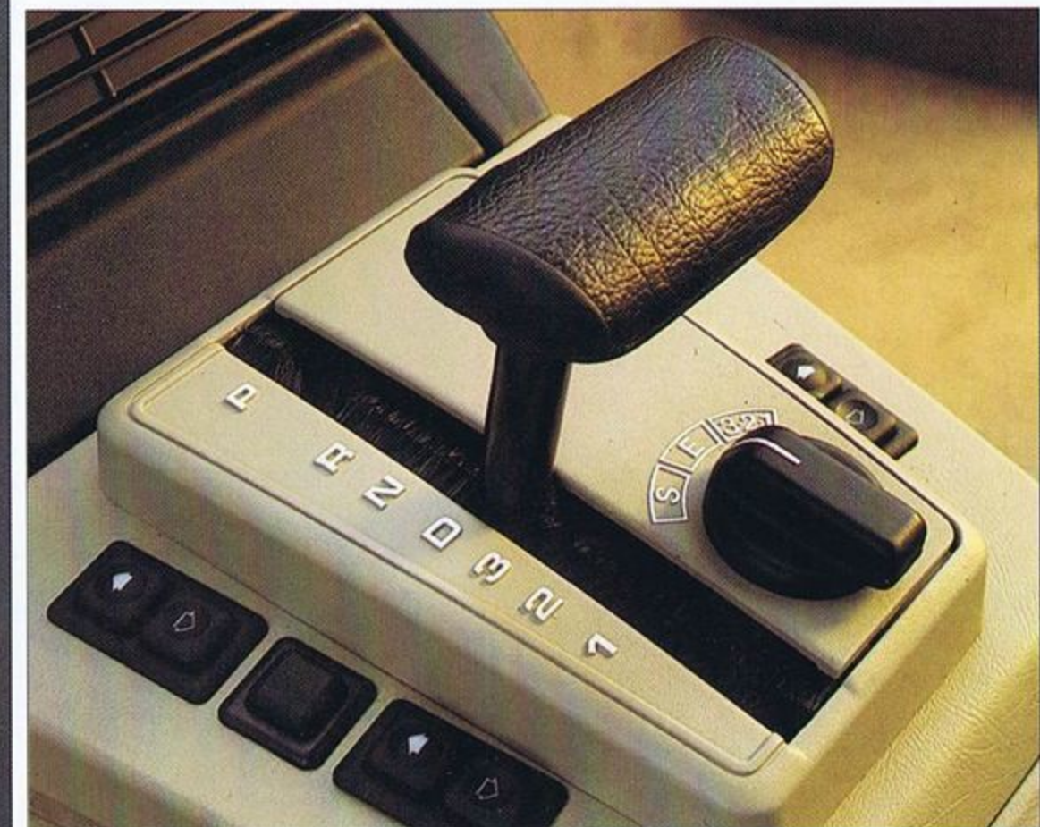
Four-speed automatic transmission (optional) with a special feature: The converter lock-up clutch provides a positive engagement of 3rd and 4th gear, ensuring absolute running smoothness without the slightest slip that takes away some of the engine power on a conventional transmission.
